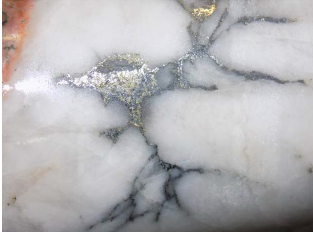
Figure 7-3 Au-Bi-Te stringers in quartz vein from 54.6 m, MG-14-12.
