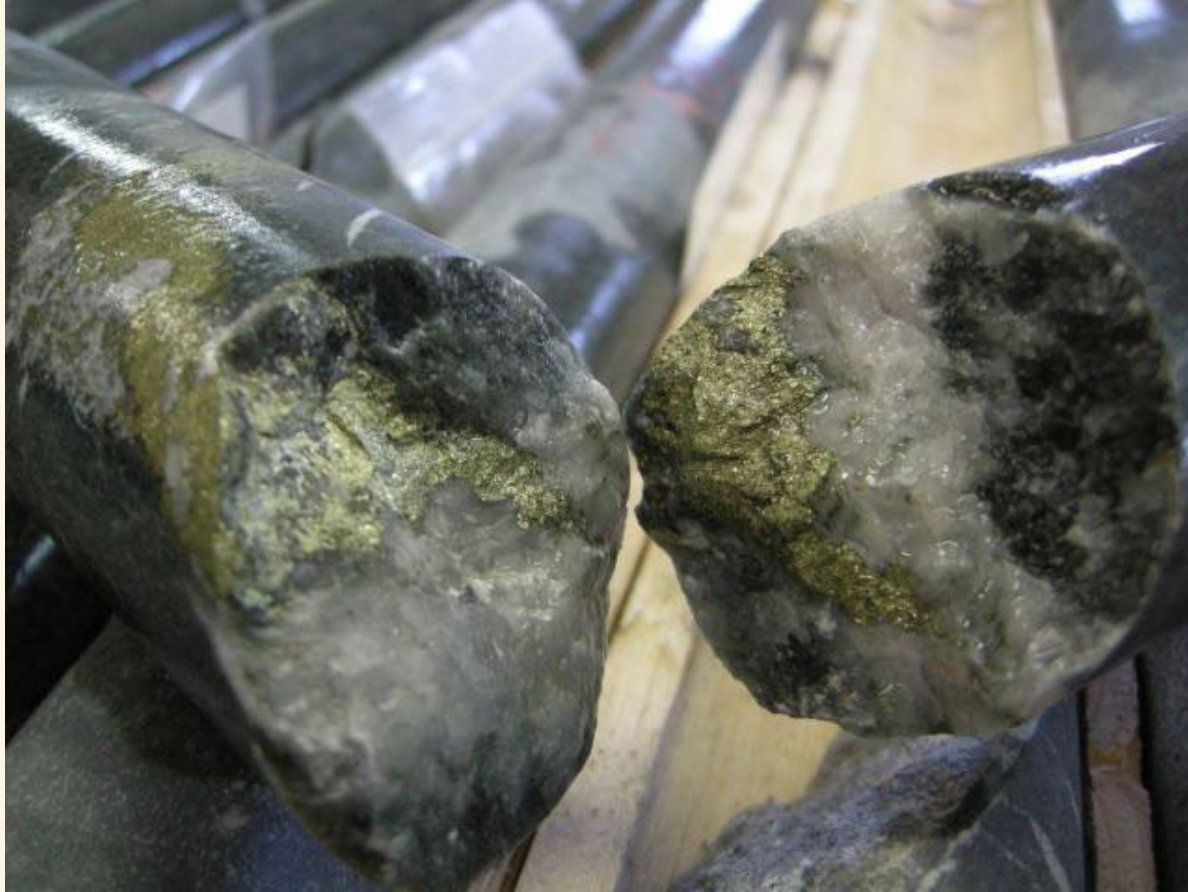
Core grading 46.5 g/t Au, 0.66% Cu over 1.0m from hole BG13-68 showing quartz vein with chalcopyrite blebs.
