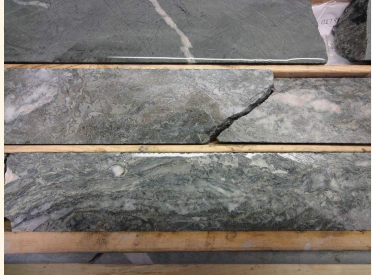
Core grading 7.89 g/t Au, 11.18 g/t Ag, 0.14% Cu and 3.77% Zn over 2.4 m from hole BG11-47 showing semi-massive pyrite and sphalerite (light grey) with pervasive silicification in mafic tuff.
