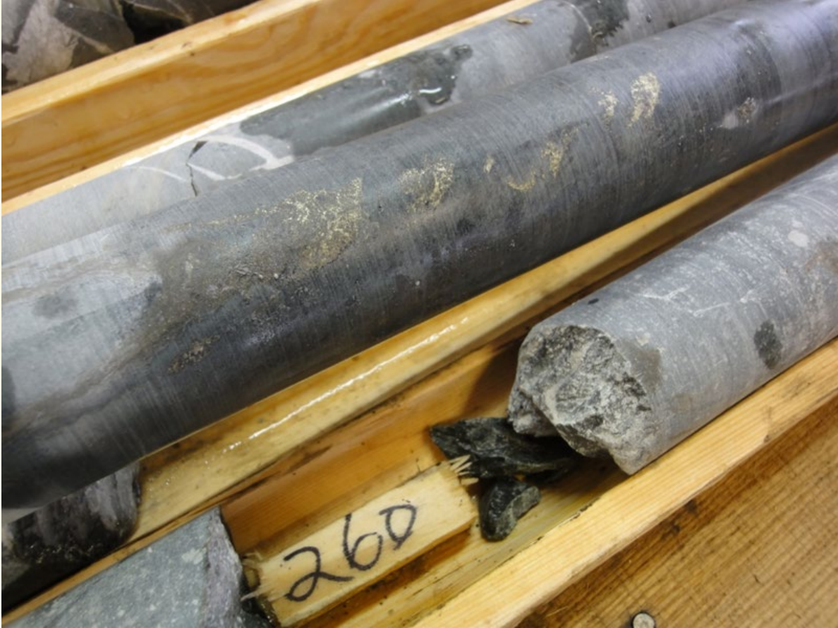
Core grading 2.09 g/t Au over 25.5m including 10.30 g/t Au over 2.0m from hole BG12-65 showing chalcopyrite stringers in intermediate porphyry.
