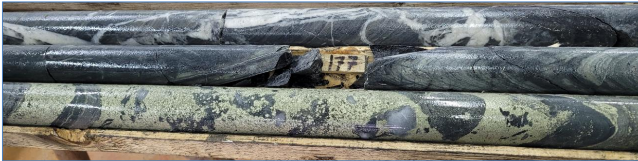
Photo 4. Zone 2 semi-massive chalcopyrite from DDH CC02-23 grading 16.05% Cu over 0.6m
