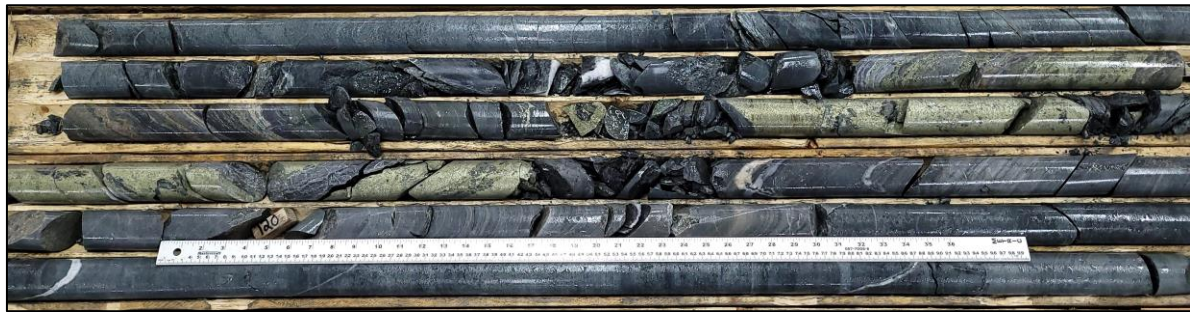
Photo 2. Zone 2 massive and stringer chalcopyrite grading 14.8% Cu over 2.45m between 116.55m and 119m in DDH CC03-23
