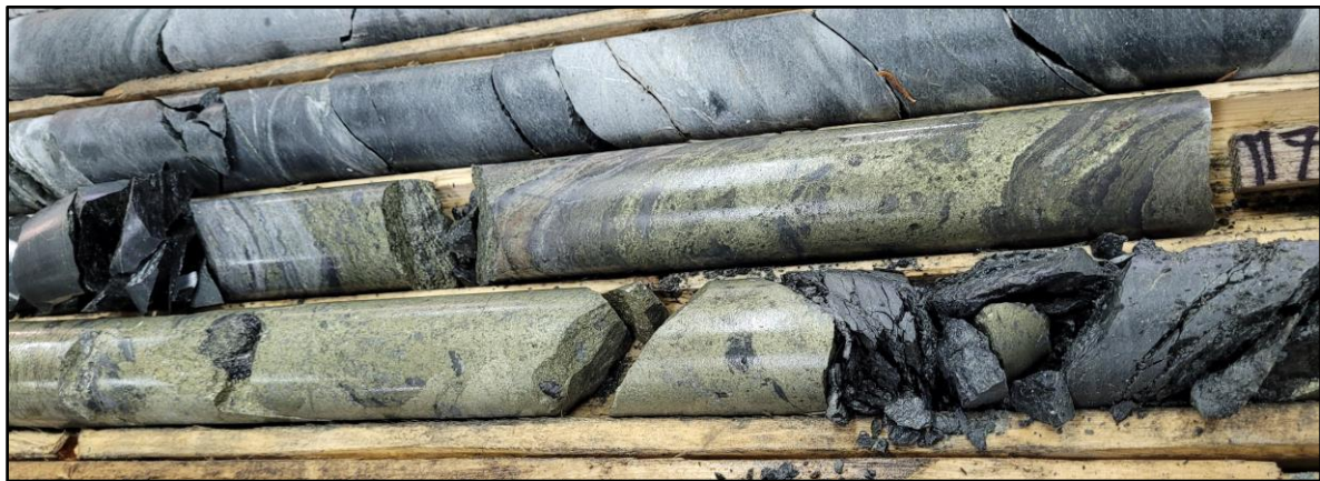
Photo 1. Massive chalcopyrite from Zone 2 grading 21.7% Cu over 1.35m in DDH CC03-23
