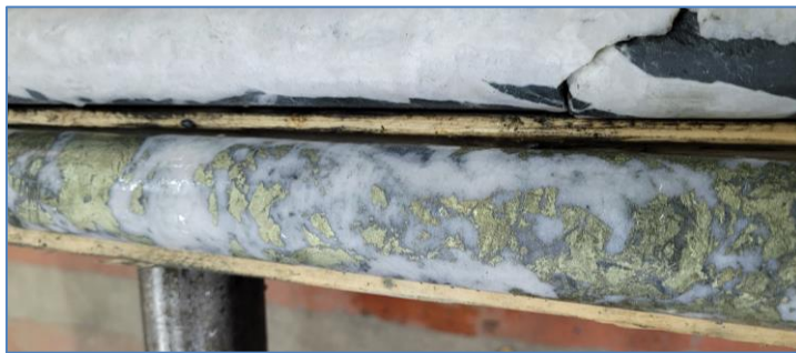
Photo 5. Zone 3 semi-massive chalcopyrite from DDH CC01-23 grading 5.91% Cu over 1.5m
