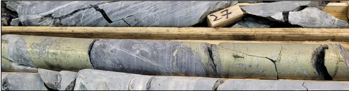
Photo 3. Zone 1 massive chalcopyrite from DDH CC01-23 grading 19.45% Cu over 0.5m
