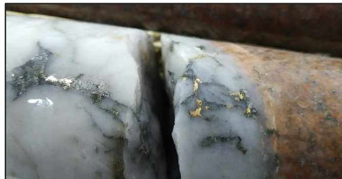
Visible Gold and Gold Tellurides @ 69.7m
