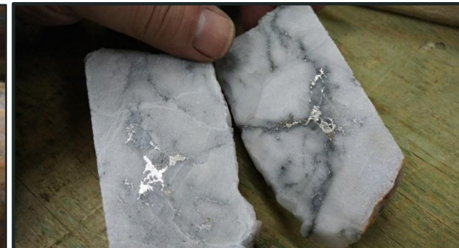
Gold Telluride Stringers @ 69.7m in Split Core
